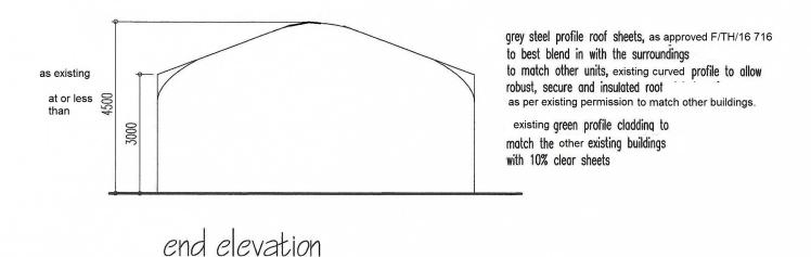
Application No. F/TH/ 20 0419 Change of Use to class E(g) Elevations for Block F (existing)
